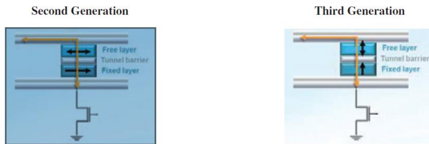
Schematic depiction of the In-Plane MTJ and Perpendicular MTJ bit cells.
